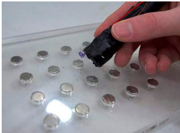
Figure 1: The Force Attraction Pen being used on a surface (in this case, a grid of magnets).
