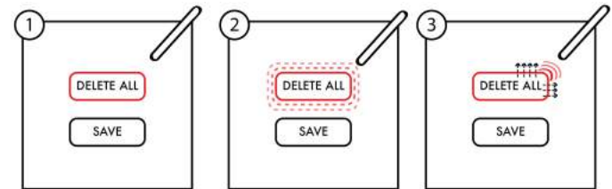
Figure 2: In this example, a “Delete All” button is surrounded by a repulsion boundary to ensure that a user must actively intend to click it. (1) The user moves freely in areas away from the “Delete All” button. (2) As the user moves the stylus closer to the “Delete All” button, the electromagnet in the stylus is polarised such that it is repelled from the grid of magnets. (3) This results in a repulsive force which offers enough resistance to prevent accidental clicking, but not so much that the user is unable to click the button if they mean to.
